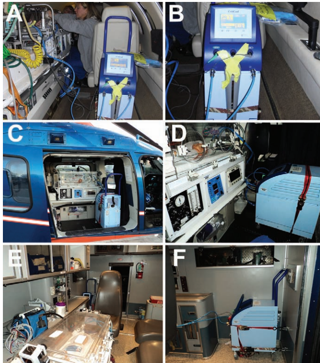
Figure 1. The CritiCool in the ambulance, fixed-wing, and helicopter. A and B demonstrate the CritiCool in our Cessna Citation. Note the yellow tape that covers the cap. C and D show the CritiCool in our Agusta A109 Power helicopter. E and F show the CritiCool in the ambulance; note in panel E the CritiCool is in the back left corner of the photograph. Note the red prototype cap in F (arrow).
